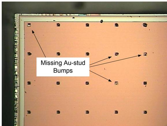
Fig. 9. A portion of the ASIC readout chip indicating locations of missing Au-stud bumps contributing to non-contact with the detector pads.
