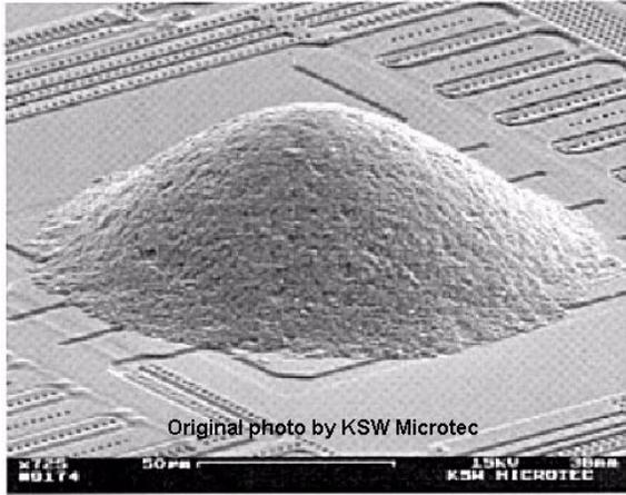
Fig. 2. Stencil printed, conductive epoxy bump (~150 $\mu$ m diameter).
