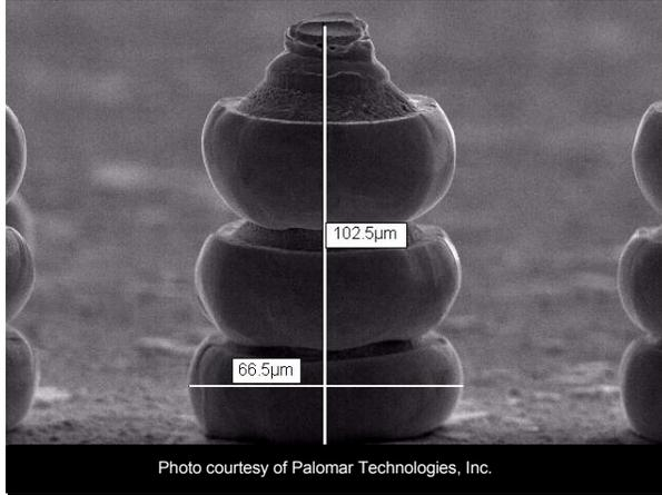
Fig. 5. SEM Photo of a triple-ball Au-stud bump.
