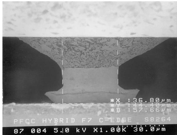
Fig. 11. SEM image of a single Au-stud bump, centered within and connecting to a silver filled, conductive epoxy bump. Note that the epoxy does not reach the surface of the bottom VLSI chip.
