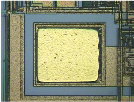
Fig. 6. Close-up photo of an electroless (Ni-Au) plated pad.
