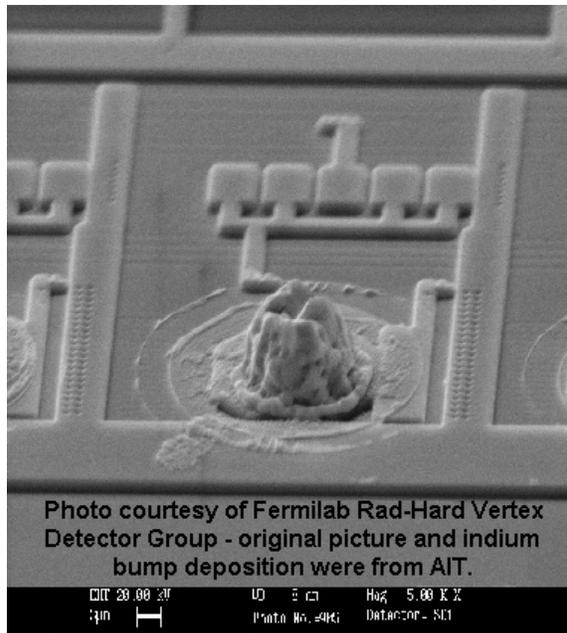
Fig. 1. SEM photo of a vacuum-deposited indium bump (~15-20 $\mu\text{m}$  diameter).
