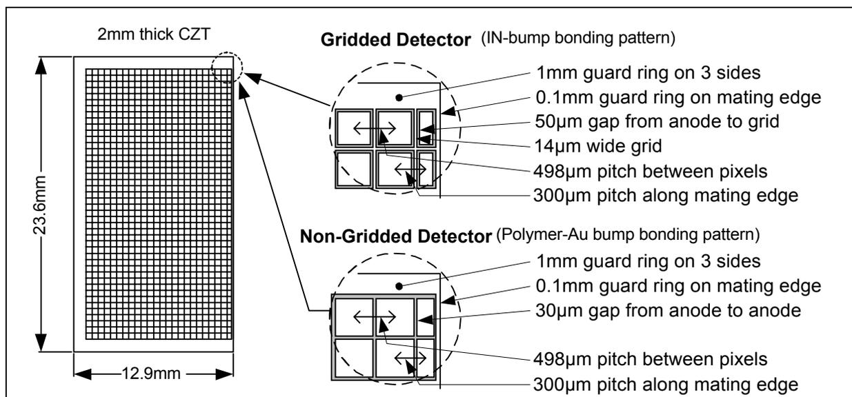
Fig. 7. Anode plane patterns. The gridded pattern at the top is designed for indium bump bonding to minimize the anode contact size and input capacitance. The no-grid pattern at the bottom is designed for bonding with conductive epoxy and gold stud bumps, which are 4-5 times taller than indium bumps. Both patterns contain a mating edge, where the last row of pixels and the guard ring are contracted for a second detector to be placed side by side.
