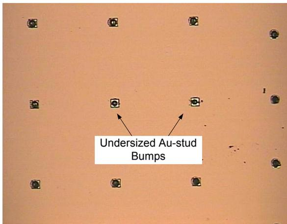
Fig. 10. A portion of the ASIC readout chip indicating locations of undersized Au-stud bumps contributing to non-contact with the detector pads.
