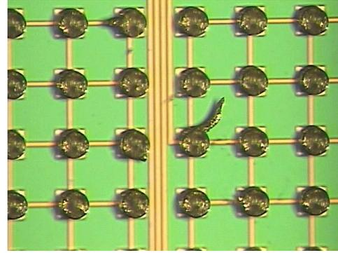
Fig. 3. Photo of Au-stud bumps with protruding wires.
