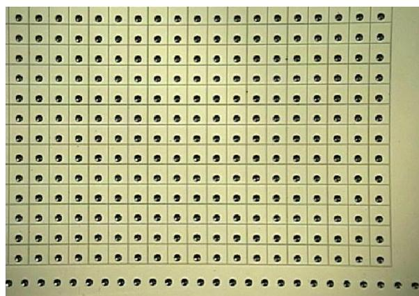
Fig. 8. A portion of a 24X44 CdZnTe pixel-array with conductive epoxy bumps spaced 498µm apart. The bumps are purposely offset from the center-point of each pixel.
