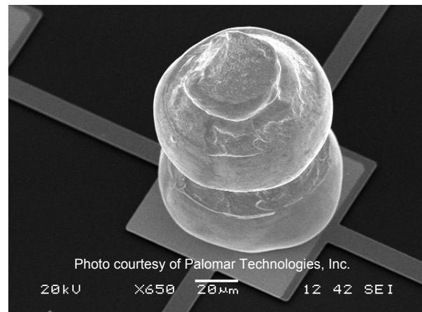
Fig. 4. SEM Photo of a double-ball Au-stud bump.
