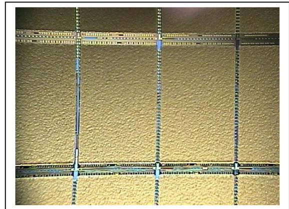
Figure 5: Wafer level epoxy screen print coating.
