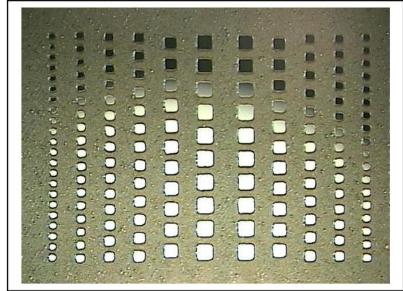
Figure 4: Wafer level epoxy coating with alpha-particle protection and thermal absorption.
